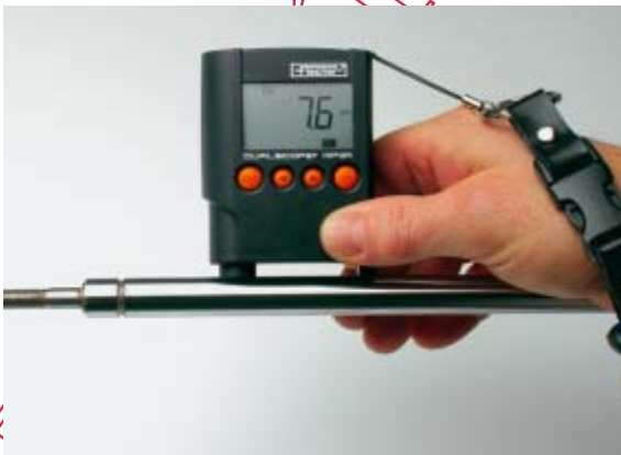
Problem-free measurements even on cylindrical parts
