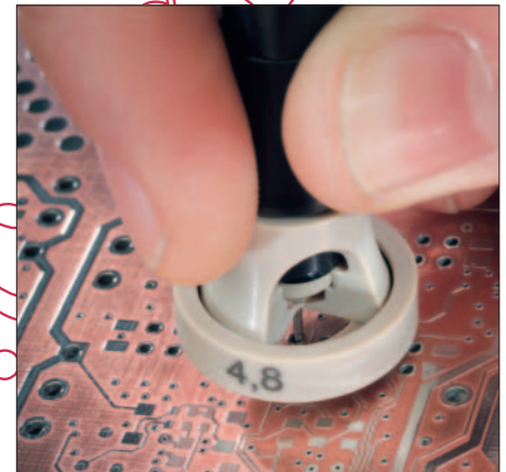
Copper cladding thickness measurement in boreholes using the probe ESL080V.
